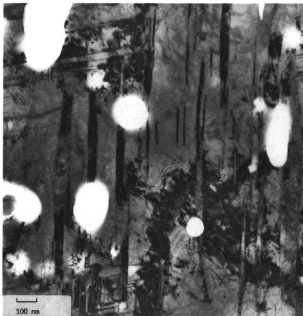
Fig. 4. TEM micrograph of a fully hydrided surface region: several single crystal hydride domains are visible separated by domain boundaries; holes are produced by the corrosive action of the acid.
